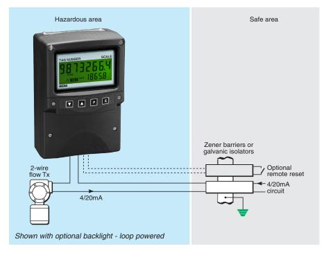
The BA354E loop powered 4/20mA rate totaliser is a third generation field mounting instrument that is electrically and mechanically compatible with the earlier BA354D, but it has a larger display, extended operating temperature and additional features such as a lineariser and bi-directional flow capabilities. Like its predecessor the BA354E is housed in a robust IP66 GRP enclosure with a separate terminal compartment.
