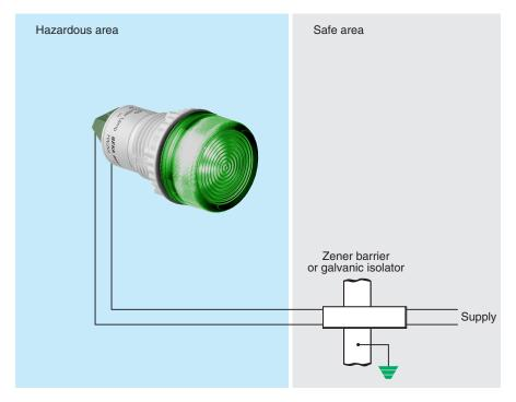
The BA390 cluster lamps provide reliable cost-effective visual status indication in all hazardous areas. Each BA390 contains a group of high efficiency light emitting diodes mounted behind a coloured diffuser to produce a bright, uniform output with a typical life greater than ten years. All models contain a 20mA current regulator which maintains constant brilliance and provides protection against excess voltages.
